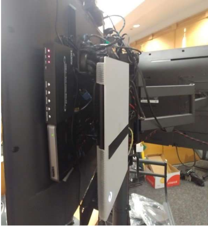
Detailed view of wireless listening devices. Devices on the left are receiving only. Devices on the right can send and receive (microphones can be attached but are not currently attached).
