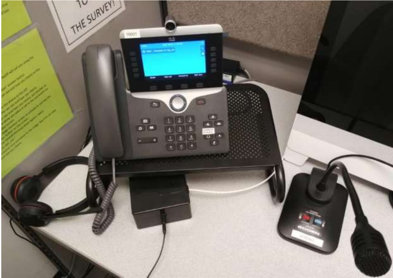
Picture of phone. Phone used to connect to the private line with the LEP, which was a second Cisco phone in the courtroom. The headphones on the headset were connected through the mixer to both the phone and DX80 for sound. The microphone on the headset was only connected to the phone. The splitter assisted with this and was provided by Paras.
