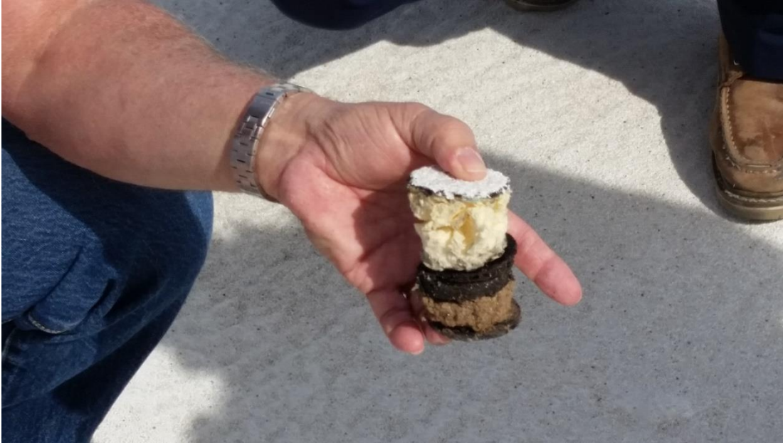
Above: Old roofing material (brown) compared to new roofing material (white) Below: Newly replaced roof
